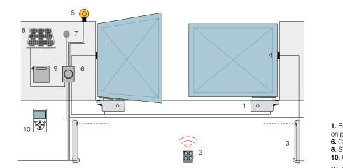
Big-Metro 2. Transmitter 3. Photocells mounted on posts 4. Photocells 5. Flashing light
